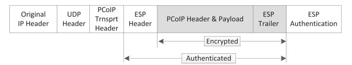
**UDP-encapsulated ESP Packet Format**
